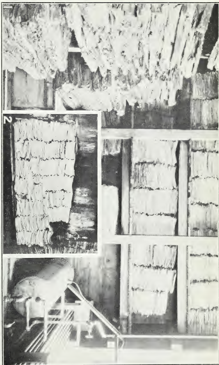
FIG. 1.—Humidity-controlled and temperature-controlled storage shed at the Forest Products Laboratory in which ground wood and sulphite pulps sprayed with 106 different chemicals were kept under observation for nearly two years. The bales in the background are in bundles of three, each being incased with five different wood-destroying fungi. The experimental pulp on the left side of the shed was incased with a large number of molds. The large bales are roll-on hydraulic-pressed ground wood used to increase the infection. Between these are single layers of bundles, each bundle consisting of seven test bales folded once. FIG. 2.—The of commercial ground-wood bales treated at a Wisconsin mill with 18 different preservatives and piled in a warm, moist basement. This experimental pulp was piled at one side against the wall and was surrounded on all other sides by the regular-run ground wood.
